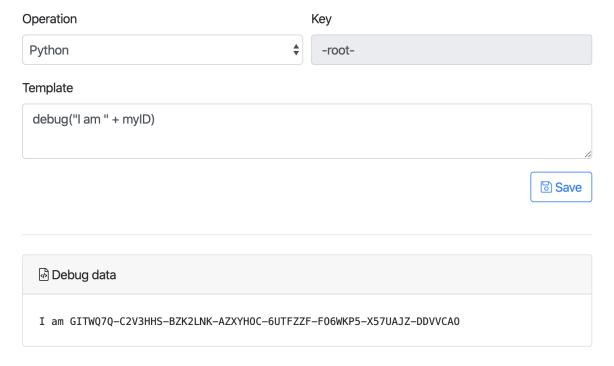
Functions and standard Python control structures can also be used to inspect and modify the configuration. One difference from standard Python is that loops and conditionals are only permitted inside functions.
